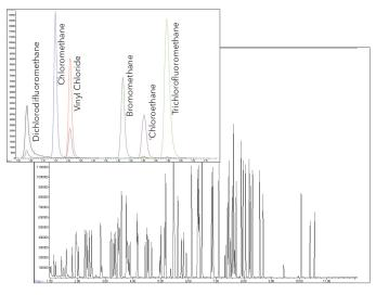
The Eclipse was used to prepare a chromatogram of an expanded list of USEPA Method 8260 standard. It illustrates superb chromatographic performance with baseline resolution for all light gases and polar compounds, even with high-speed columns.
